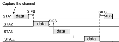
Fig. 4. Active/idle switching diagram of the mobile devices in one cluster
